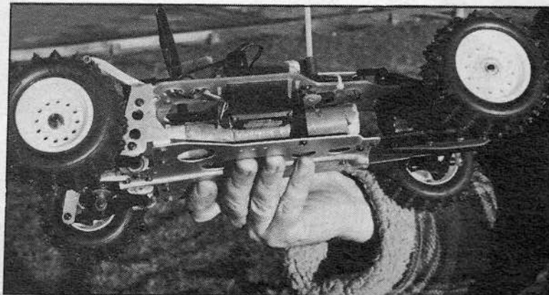
Above: Steve Newey's modified 'Progress', note the heavy components: speed controller and Ni-Cads, mounted between the chassis and radio plate as low as possible to lower the CoG. The rear dampers' top mounting point is provided by some suitably formed alloy section taken from an old 'Scorpion' chassis. Right: the Ni-Cad pack is now positioned lengthways along the chassis.
